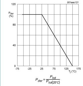
Fig. 2. Normalized total power dissipation as a function of junction temperature
