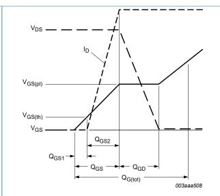
Fig. 16. Gate charge waveform definitions
