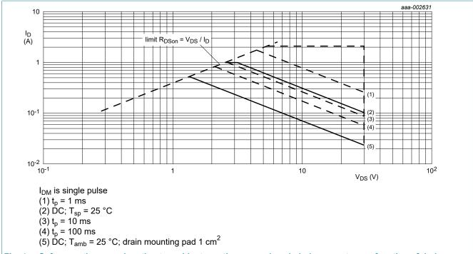
Fig. 4. Safe operating area; junction to ambient; continuous and peak drain currents as a function of drain-source voltage
