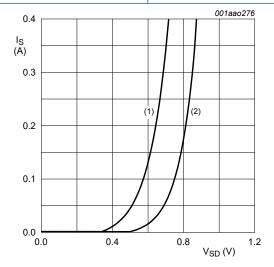
$V_{GS} = 0 V$ (1)  $T_j = 150 \,^{\circ}C$ (2)  $T_j = 25 \,^{\circ}C$
