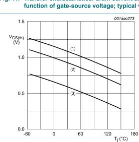
$I_D = 0.25 \text{ mA}; V_{DS} = V_{GS}$
